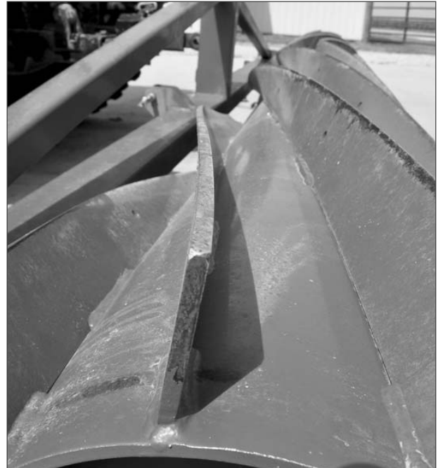
The Chevron-pattern on the crimp roller prevents soil disturbance and reduces vibration in the tractor. The blunt edges snap the rye stem without cutting it.
